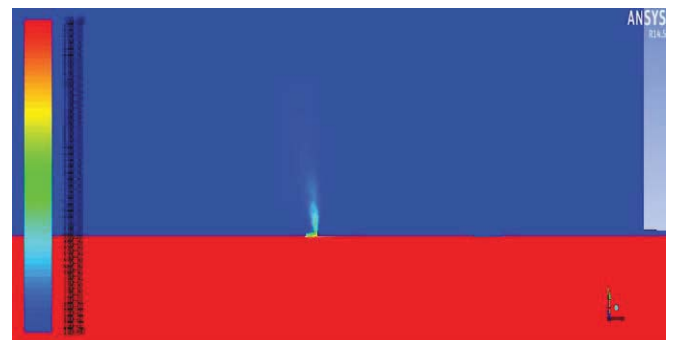
Fig. 6 Contours of mass fraction of CH 4 with mass flow rate 0kg/s and hole diameter 5cm
