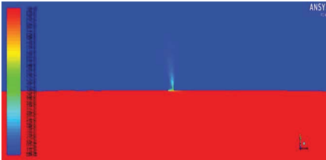
Figure 4: contours of mass fraction of methane at wind velocity 0m/s
